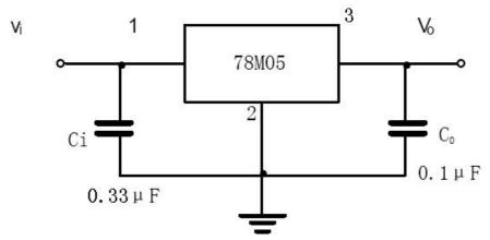
\*Bypass capacitors are recommended for optimum stability and transient response and should be located as close as Possible to the regulators.
